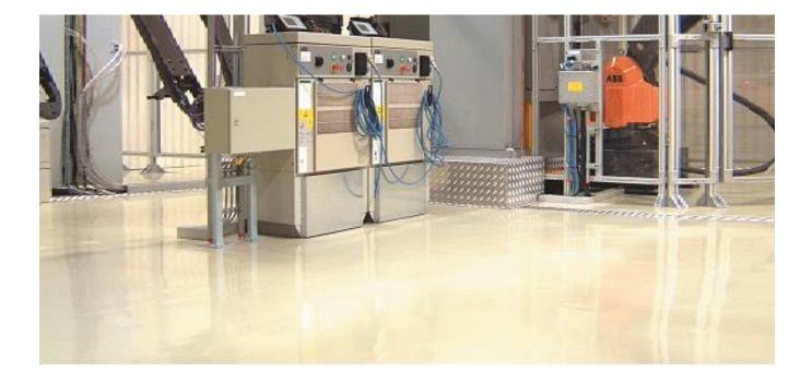
Eradur® ESD Resistant LM3 is a chemical resistant epoxy coating with anti-static properties, ie the coating dissipates static electricity and counteracts sparking.
